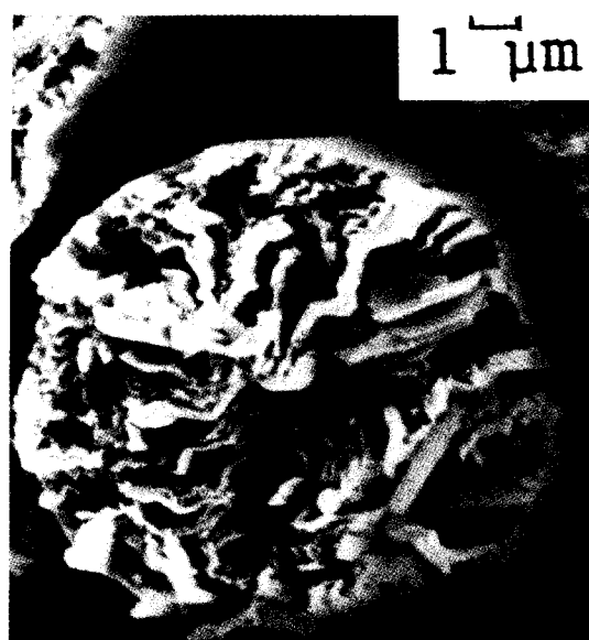
Fig. 7. SEM photograph of a Type I du Pont E-130 fiber, showing the cross-sectional view.
